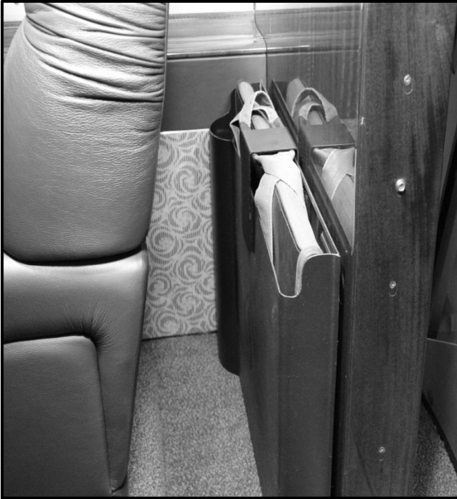
Storage Case mounted horizontally on forward cabin bulkhead behind passenger
