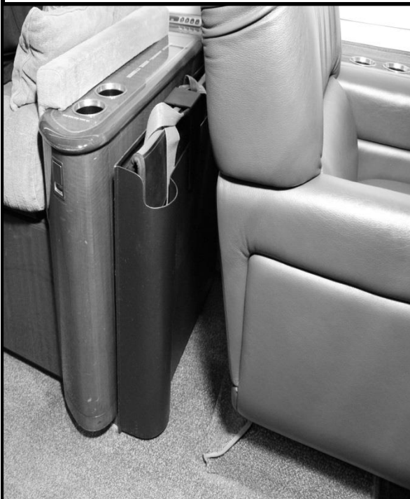
Storage Case mounted horizontally on forward Divan cabinet behind
