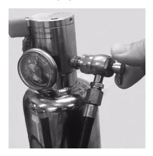
Remove the protective valve cap from suppression system and install included depressurization tool on Schrader valve fitting.
